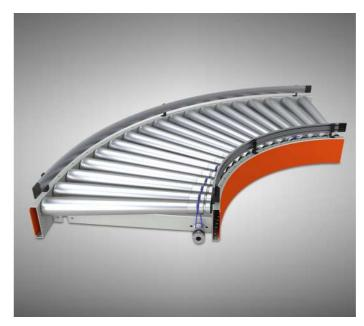
The curve with royal shaft changes the direction of movement of the load. The conical shape of the rollers keeps objects between the side profiles. The curve connected to the driven module forms the lineshaft system. The device consists of a steel frame bent at an angle of 90°, rollers, shafts, PU straps and blends.
