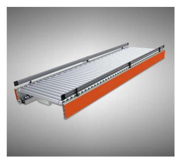
Driven lineshaft is a conveyor driven by a royal shaft, which mediates in the drive of rollers by the engine. The drive module is a segment equipped with its own drive. It is a basic module that is connected to passive segments, curves and angle connectors in any configuration. The device consists of a steel frame, rollers, shaft, PU belts, motor and blends.
