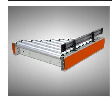
The roller infeed, depending on the location, helps to put loads on the main line or lead them to the side line. With the angle of inclination of this section, the speed of transported objects increases. The device consists of a steel frame shaped at an angle of 45°, straight gravity rollers and plastic covers.
