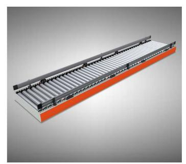
Zone conveyor supports the accumulation of objects in more complex lines. Each zone in the roller conveyor is programmed separately, which gives the possibility to adjust the speed and functionality of the zone. The conveyors are fully compatible with specialized devices such as transfers, divertors and pop-up modules. The device consists of a steel frame, electric rollers, PolyVee rollers, belts, controllers, sensors and blends
