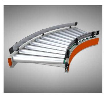
The gravitational curve changes the direction of movement of the object. Can be installed at an angle or horizontally. When set at an angle, the speed of transported objects increases in proportion to the degree of inclination. The device consists of a steel frame bent at an angle of 60°, twelve tapered rollers and a plastic cover.
