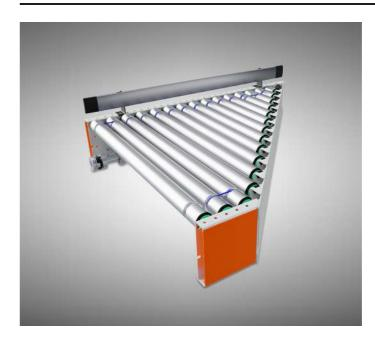
The angle connector, depending on the location, helps to put loads on the main line or lead them to the side line. Connected with the drive module, they form a lineshaft system. The device consists of a steel frame shaped at an angle of 45°, rollers, shaft, PU strips and blends.
