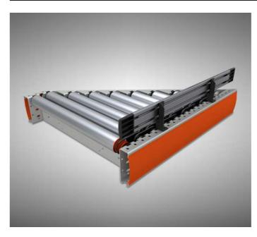
The angle connector, depending on the location, helps to put loads on the main line or lead them to the side line. When entering the main line, it uses gaps in the flow of materials. Directly works with a crossover or pop-up. The device consists of a steel frame shaped at an angle of 45°, electric roller, PolyVee rollers, belts, controller, sensor and blend.
