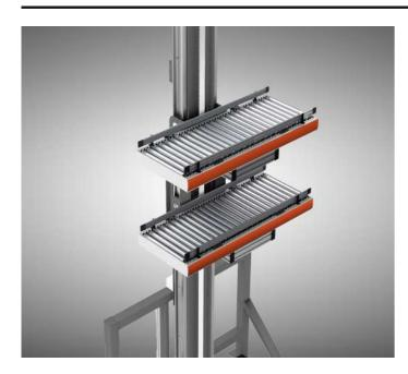
Vertical lift allows to transport goods vertically on maximum four levels. All lifts are individually designed according to customer requirements. Carriages are fully configurable in terms of width, number of zones and band height. The devices are offered in a set containing: stand, lift pole and carriage - zone conveyors.
