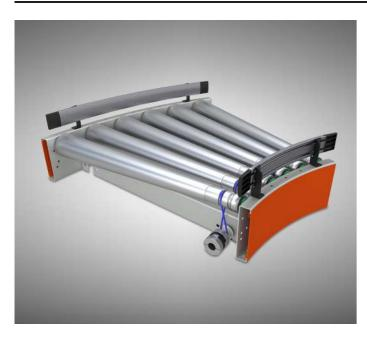
The curve with royal shaft changes the direction of movement of the load. The conical shape of the rollers keeps objects between the side profiles. The curve connected to the driven module forms the lineshaft system. The device consists of a steel frame bent at an angle of 30°, rollers, shafts, PU straps and blends.
