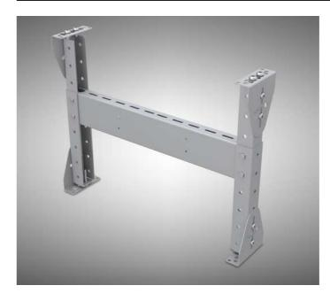
A support is intended for fixing conveyors to the ground. Available height is in the range of 480 - 2000 mm with additional calibration useful to compensate for uneven ground. It is made of galvanized steel. The light support can be used in all types of conveyors.
