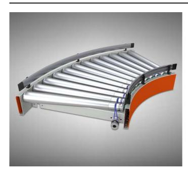
The curve with royal shaft changes the direction of movement of the load. The conical shape of the rollers keeps objects between the side profiles. The curve connected to the driven module forms the lineshaft system. The device consists of a steel frame bent at an angle of 60°, rollers, shafts, PU straps and blends.
