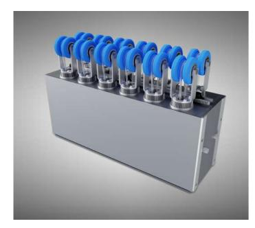
The diverter is used to direct objects to lines at an angle of 30°, 45° or 90°. Loads are redirected according to the setting of the rotary rollers. In some cases, it is possible to change the orientation of an object by 90°.
