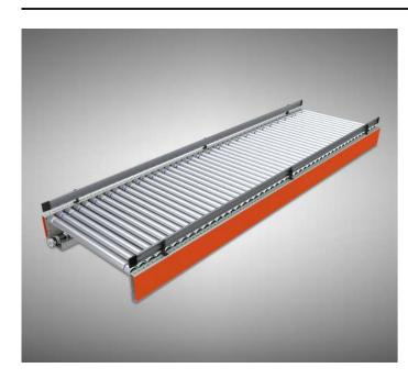
Passive Lineshaft is a segment that is not equipped with a drive. Several passive modules connected together with the drive module form the lineshaft system lines. The device consists of a steel frame, rollers, shaft, PU strips and blends.
