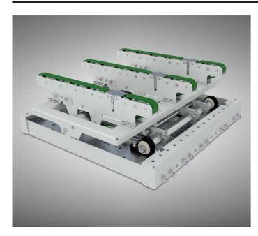
The basic function of belt transfers used in warehouse automation systems is to shift the load between parallel or perpendicular lines (picking stations). Objects are lifted by means of an electric motor and then shifted to the side line by means of transmission belts. The load is transferred perpendicularly to the direction of travel with the simultaneous change of its orientation by 90°.
