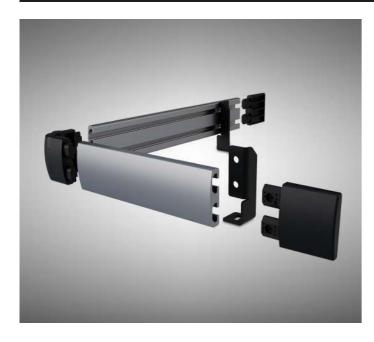
The bands are used to secure the transported product against sliding off the conveyor line. We offer aluminum bands with polymer endings. We adapt the profile by rolling on sections of curves, connecting and direction-changing nodes to ensure the correct flow of cargo. The top edge of the band is about 90  $\mbox{mm}$ above the conveyor.
