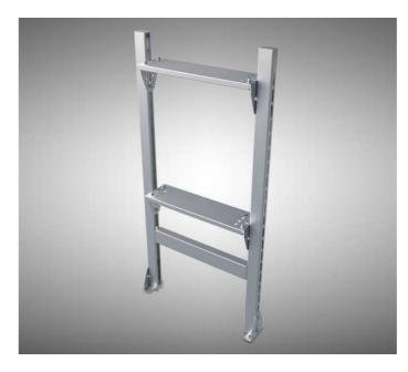
Storey support is intended for fixing conveyors to the ground. Available height 2000 mm with additional calibration useful to compensate for uneven ground. The support is made of galvanized steel. Heavy supports are used in the two or three storeyed lines.
