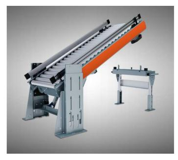
Driven zone gate enables free passage through the conveyor main line. Raising the gate stops the transported loads until its put down back. It consists of a steel conveyor frame, electric rollers, PolyVee rollers, controllers, sensors, lifting system and blends.
