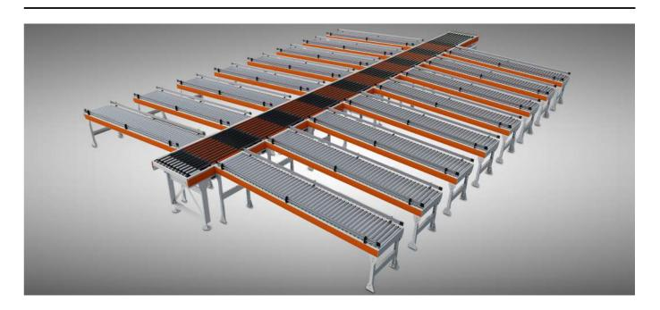
Narrow Belt Sorter uses a set of narrow straps to carry the product over the sorter's surface. In addition, the sorter is equipped with high-friction rollers to enable the dropping of goods. They allow the goods to be picked up from the conveyor for redirection under the 90° account to the right or left. The continuous contact of the belt with the product ensures maximum guidance accuracy, which affects the sorting reliability.
