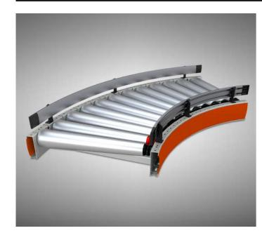
The roller curve changes the direction of cargo movement. The conical shape of the rollers allows the goods to be kept between the side profiles. The use of a controller enables no-pushing buffering. The device consists of a steel frame bent at an angle of 60°, electric roller, eleven PolyVee tapered rollers, belts, controller, sensor and blends.
