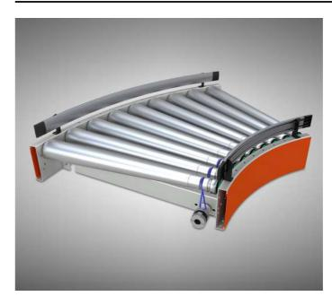
The curve with royal shaft changes the direction of movement of the load. The conical shape of the rollers keeps objects between the side profiles. The curve connected to the driven module forms the lineshaft system. The device consists of a steel frame bent at an angle of 45°, rollers, shafts, PU straps and blends.
