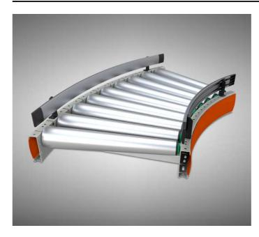
The gravitational curve changes the direction of movement of the object. Can be installed at an angle or horizontally. When set at an angle, the speed of transported objects increases in proportion to the degree of inclination. The device consists of a steel frame bent at an angle of 45°, nine tapered rollers and a plastic cover.
