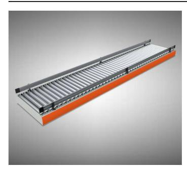
The non-driven straight section of the gravity conveyor can be installed at an angle or horizontally. When set at an angle, the speed of the transported objects increases with the inclination to the ground. The device consists of a steel frame, simple gravity rollers and blends.
