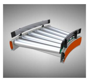
The gravitational curve changes the direction of movement of the object. Can be installed at an angle or horizontally. When set at an angle, the speed of transported objects increases inproportion to the degree of inclination. The device consists of a steel frame bent at an angle of 30°, six tapered rollers and a plastic cover.
