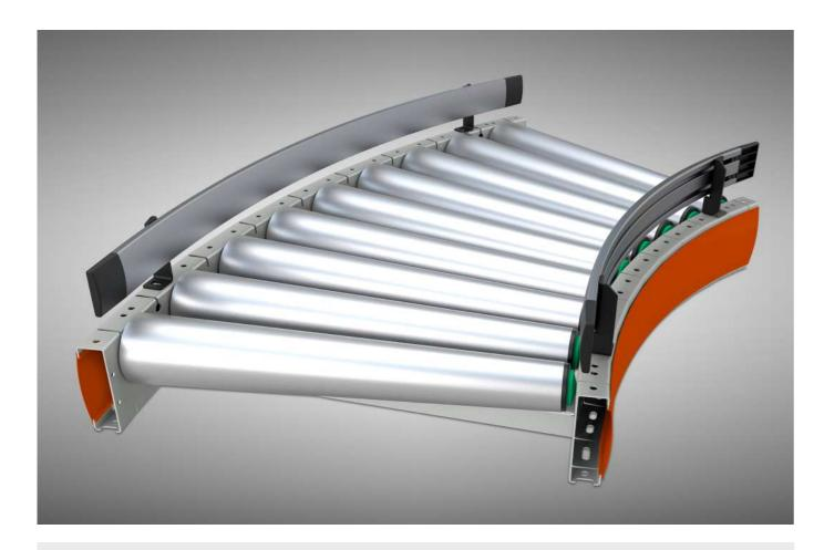
Gravity roller conveyors do not have their own drive source. Loads are moved due to their own weight and a properly selected angle of inclination - thanks to the force of gravity and manual shifting - manual force. Devices of this type are often used as buffers on transport lines, connectors and end stations. The systems with various angles and angle connectors give great freedom in configuring the systems.
