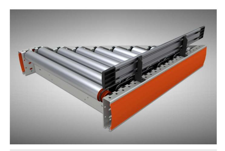
24V conveyors are driven by electric rollers connected by means of multi V-belts with other rollers. The design of this type of equipment allows it to be configured with other systems such as gravity conveyors, belt conveyors, transfers, switches and pop-up modules. Together with the extensive sensor system, they form a fully automated internal transport system.
