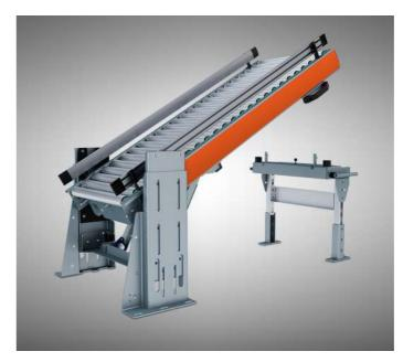
Lifted conveyor gate allows free passage through the conveyor main line. Lifting the gate stops transported loads until it is put down. The device consists of a steel frame of the conveyor, straight gravity rollers, lifting system and plastic covers.
