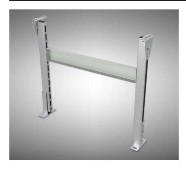
The support is intended for fixing conveyors to the ground. Available height in the range of 480 - 2000 mm with additional calibration useful to compensate for uneven ground. The heavy support is covered with a varnish coat. Heavy support can be used in each type of conveyors, especially in heavy load lines.
