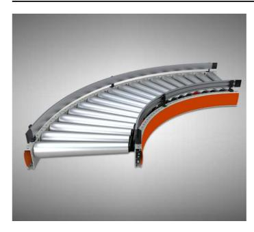
The roller curve changes the direction of cargo movement. The conical shape of the rollers allows the goods to be kept between the side profiles. The use of a controller enables no-pushing buffering. The device consists of a steel frame bent at an angle of 90°, two electric roller, seventeen PolyVee tapered rollers, belts, controller, sensor and blends.
