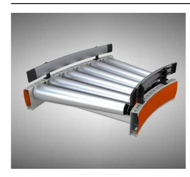
The roller curve changes the direction of cargo movement. The conical shape of the rollers allows the goods to be kept between the side profiles. The use of a controller enables no-pushing buffering. The device consists of a steel frame bent at an angle of 30°, electric roller, five PolyVee tapered rollers, belts, controller, sensor and blends
