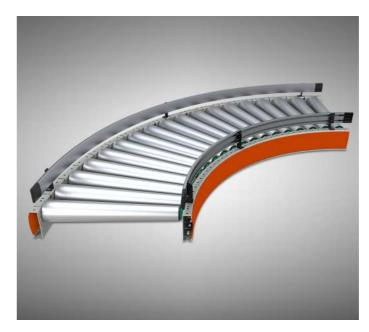
The gravitational curve changes the direction of movement of the object. Can be installed at an angle or horizontally. When set at an angle, the speed of transported objects increases in proportion to the degree of inclination. The device consists of a steel frame bent at an angle of 90°, eighteen tapered rollers and a plastic cover.
