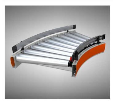
The roller curve changes the direction of cargo movement. The conical shape of the rollers allows the goods to be kept between the side profiles. The use of a controller enables no-pushing buffering. The device consists of a steel frame bent at an angle of 45°, electric roller, eight PolyVee tapered rollers, belts, controller, sensor and blends.
