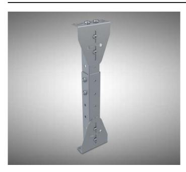
A single support is intended for fixing conveyors to the ground. Available height is in the range of 480 - 2000 mm with additional calibration useful to compensate for uneven ground. It is made of galvanized steel. The single support is used for angular entrances and  $60^\circ, 90^\circ$  arches.
