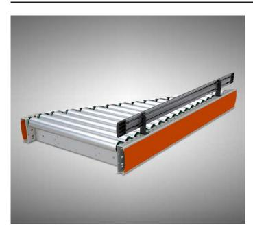
The roller infeed, depending on the location, helps to put loads on the main line or lead them to the side line. With the angle of inclination of this section, the speed of transported objects increases. The device consists of a steel frame shaped at an angle of  $30^\circ$ , straight gravity rollers and plastic covers.
