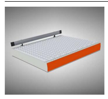
Ball transfer table helps to move products in any direction with little force. Mainly used at inspection or picking stations. The device consists of a steel frame, laminated chipboard, transport bearings and plastic covers.
