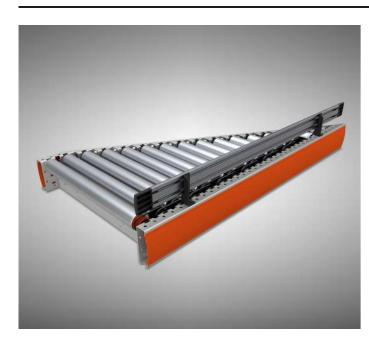
The angle connector, depending on the location, helps to put loads on the main line or lead them to the side line. When entering the main line, it uses gaps in the flow of materials. Directly works with a diverter or pop-up. The device consists of a steel frame shaped at an angle of 30°, electric roller, PolyVee rollers, belts, controller, sensor and blend.
