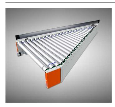
The lineshaft infeed depending on the location, helps to put loads on the main line or lead them to the side line. Connected with the drive module, they form a lineshaft system. The device consists of a steel frame shaped at an angle of 30°, rollers, shaft, PU straps and blends.
