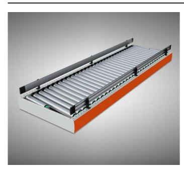
Positioning roller conveyor positions the item to the selected side in the band's profile. It is used when precision is required when changing the direction of movement of the transported load. It is recommended to place the leveling conveyor in front of the node equipped with specialized devices. The device consists of a steel frame, electric rollers, PolyVee rollers, belts, controllers, sensors and blends.
