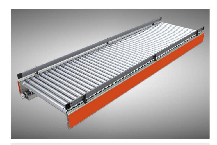
The lineshaft conveyor is a simple and very popular solution for transporting loads. The system requires a small number of drives, which significantly reduces the cost of the conveyor. One gearmotor can drive a line up to 15 meters long.
